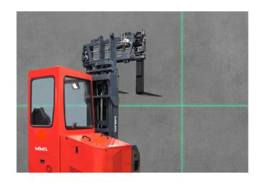
The MiMA multi-directional counterbalance forklift features an advanced laser system that enhances precision by projecting a guide onto both the ground and walls simultaneously, ensuring precise load placement in compact spaces.
