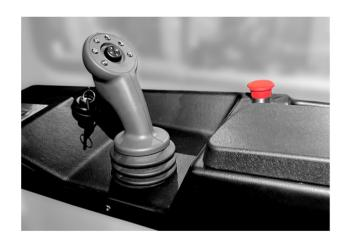
The MiMA multi-directional counterbalance forklift is equipped with integrated joystick control, offering intuitive and precise manoeuvering. This ergonomic feature enhances operator comfort and efficiency, facilitating seamless navigation in diverse material handling environments.
